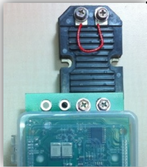
13kV SiC MOSFET based SST with Inductor (4mH) integrated coaxial winding transformer
