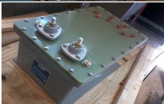
70kVA, 10kHz, 22kV/11kV/800V Transformer
