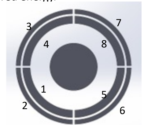
Winding order of optimal 8-turn, 2 layer winding
