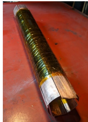
Second composite tube prior to transformer assembly
