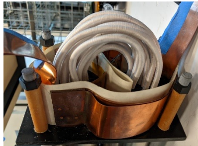
Detail of foil end connections, insulation, and primary Litz winding
