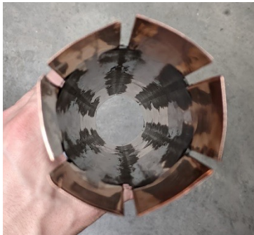
Composite winding tube has direct copper-air cooling
